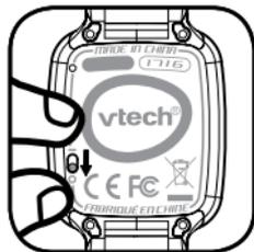
2. Loosen the four screws on the back of the watch using a cross head screwdriver, then remove the back.
